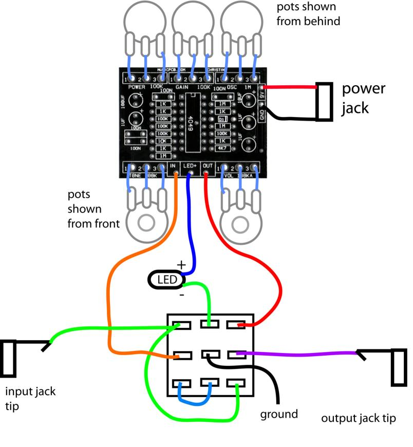
Tie switch ground and input/output jack grounds to power jack negative tab
